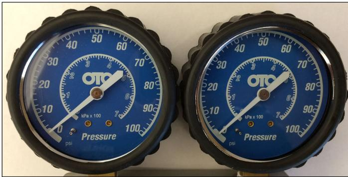
Figure 2. Dual Gauge Leakdown Test Tool.
