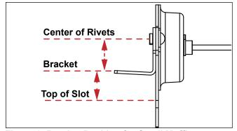
Figure 2. Bracket Position for Small Muffler.
