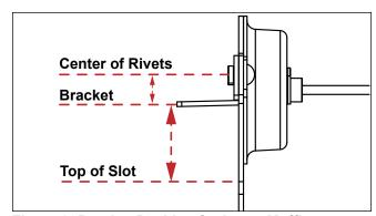
Figure 3. Bracket Position for Large Muffler.
